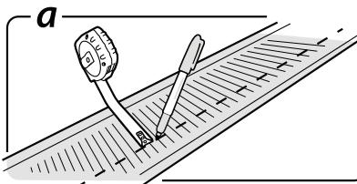
**MEASURE & MARK:** Measure the length from the lip of the gutter to the fascia board. Using that measurement, mark a line on the gutter guard where you will bend the mesh.
