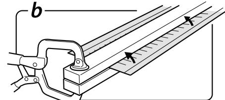
**CLAMP MESH:** Clamp the gutter guard between two 1 IN. x 2 IN. boards to hold it
