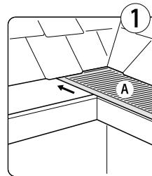
Slide piece A into the inside corner of your gutter.
