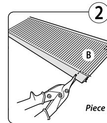
For piece B, trim back the aluminum rail about 1IN., leaving some mesh exposed.
