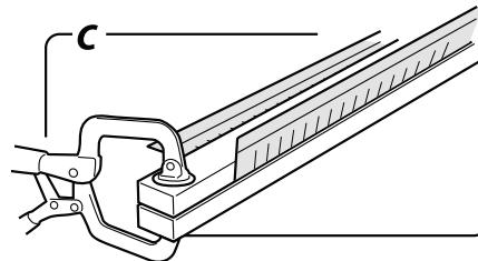
**BEND THE MESH:** Use the leverage from the clamp and/or boards to bend the mesh along the line you've marked.
