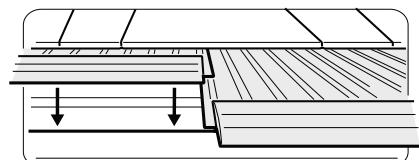
Lay one end of the mesh so it overlaps directly over the other section.
