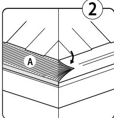
Bend down the aluminum rail and mesh to create a 45° angle.
