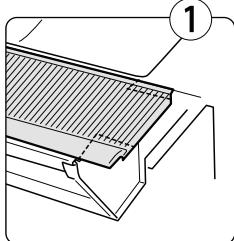
At the end of a stretch of gutter, mark on each aluminum rail where it meets the end of the gutter.
