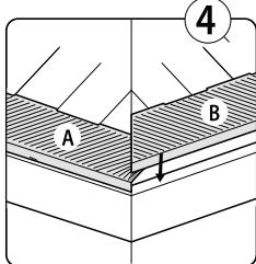
Once cut, fit it into the outside edge so that it's aligned with piece A.
