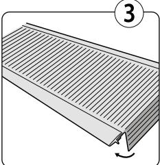
Bend and tuck the exposed mesh into the gutter. You can trim the mesh as needed to create a good covering.
