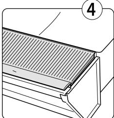
Make sure the entire gutter end is sealed to prevent debris from getting under the gutter guards.
