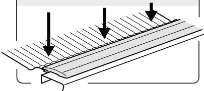
Mesh trough should be at least 1/8 IN. below gutter lip. Use fingers to push mesh trough down.
