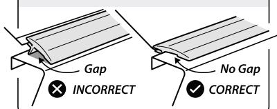
There should be no space between the front rail and the gutter lip when you install.
