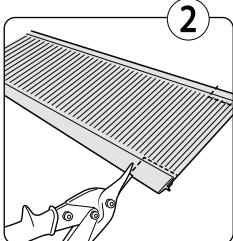
From the ground, trim back the aluminum rails where they are marked to expose the remaining mesh.
