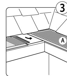
Tuck the exposed mesh of piece B down inside the gutter adjacent to the adjoining gutter guard.
