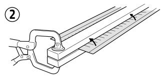
**BEND THE MESH:** Bend the mesh up or down, depending on your installation method, using a commercial or custom wooden brake.
