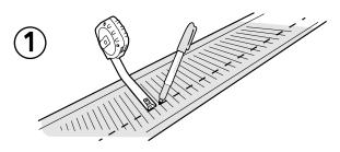
**MEASURE & MARK:** Measure and mark on the miter section where to place the bend in the mesh
