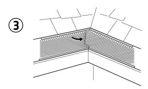
**INSTALL GUARDS:** Place the first pre-cut side of the miter into the corner of the gutter. Overlay the second side, making sure the two sections meet flush at the front corner. The mesh will overlap approximately 2 inches in the center.
