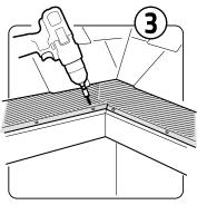
Once both sections are in place, screw the front rail of each section to the front lip of the gutter using 2 screws per section.
