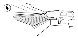
**SCREW IT DOWN:** Once both sections are in place and properly sloped, screw the front rail of each section to the front lip of the gutter, and the back rail, or mesh, to the fascia.
