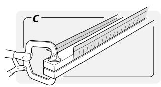
**BEND THE MESH:** Use the leverage from the clamp and/or boards to bend the mesh along the line you've marked. Note: Bend the mesh either up or down depending on your qutter-to-roof scenario.
