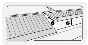
Carefully slide the rear rail of the gutter guard under the roof shingles. Continue to step 5.
