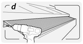
**INSTALL GUARDS:** Screw the mesh to the fascia board using 3 screws per section. Continue to step 5.
