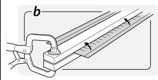
**CLAMP MESH:** Clamp the gutter guard between two 1"x2" boards to hold it in place.
