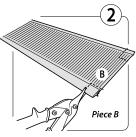
For piece B, trim back the aluminum rail about 1", leaving so mesh exposed.
