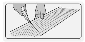
Use a new, or freshly sharpened, pair of tin snips to cut through the aluminum rail and mesh.
