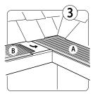
Tuck the exposed mesh of piece B n inside the gutter adjacen to the adjoining gutter guard.
