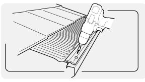
**SCREW IT DOWN:** Use the guides on the front rail to place the screw. Fasten with 3 screws for each section.
