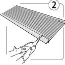
From the ground, trim back the aluminum rails where they are marked to expose the remaining mesh.
