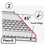
Cut the end of adjoining Piece B at 45-degrees. Repeat the 1/2 IN. wide notch cut on the back wing and the 3/4–1 IN. trim from the front edge. Pieces A & B should slightly overlap.
